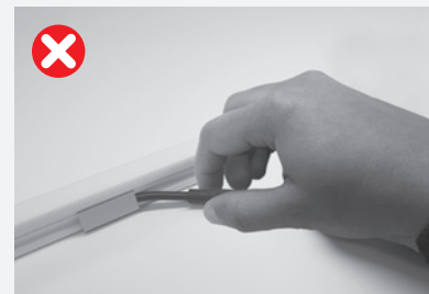
DO NOT tug cable connector or integral cable clamp assembly - excessive tension may cause malfunction or affect IP67 integrity.
